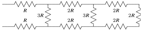
8. Find the potential difference across each of the resistors in the following circuit.
