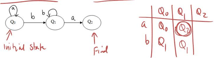
• The FSM can be in any one of the states and can transit from one state to another based on a series of rules given by a transition function.
