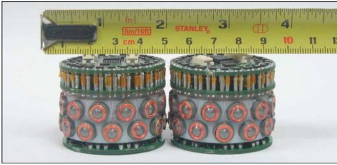
Figure 5. 44mm "Catom" modules [5]
