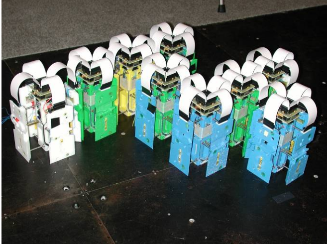
Figure 2. A set of crystalline atoms. Each is 50cm per side when contracted. [8]
