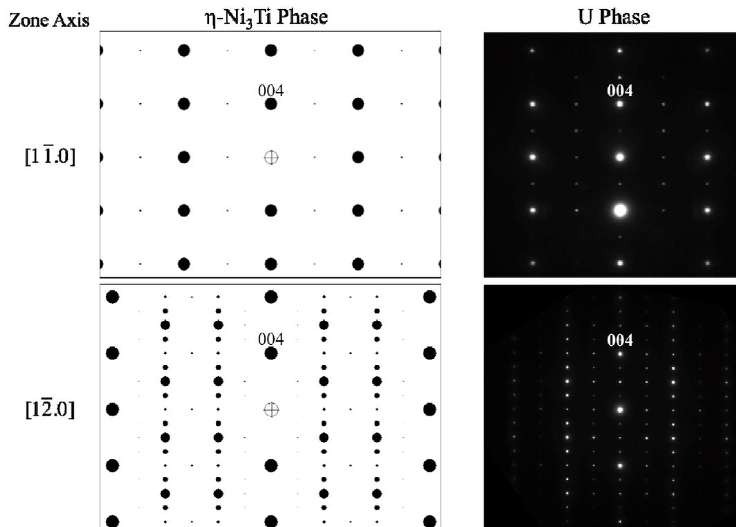
Fig. 8 Comparing simulated diffraction patterns for the  $\eta\text{-Ni}_3\text{Ti}$  phase and the experimental diffraction patterns obtained at zone axes orientations of  $[1\bar{1}.0]$  and  $[1\bar{2}.0]$ .
