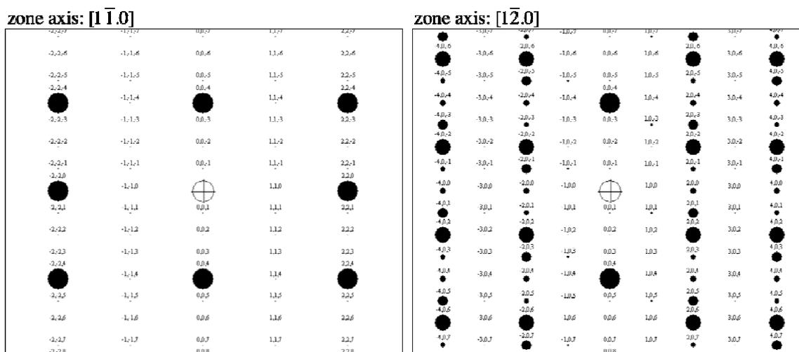
Fig. 9 Simulated  $[1\bar{1}0]$  and  $[1\bar{2}0]$  zone axis diffraction pattern for substitution of any one of the 16 sites in the unit cell of  $\eta$  phase by a Ta atom. (The spots that are labeled by plane indices are the ones allowed for the structure)
