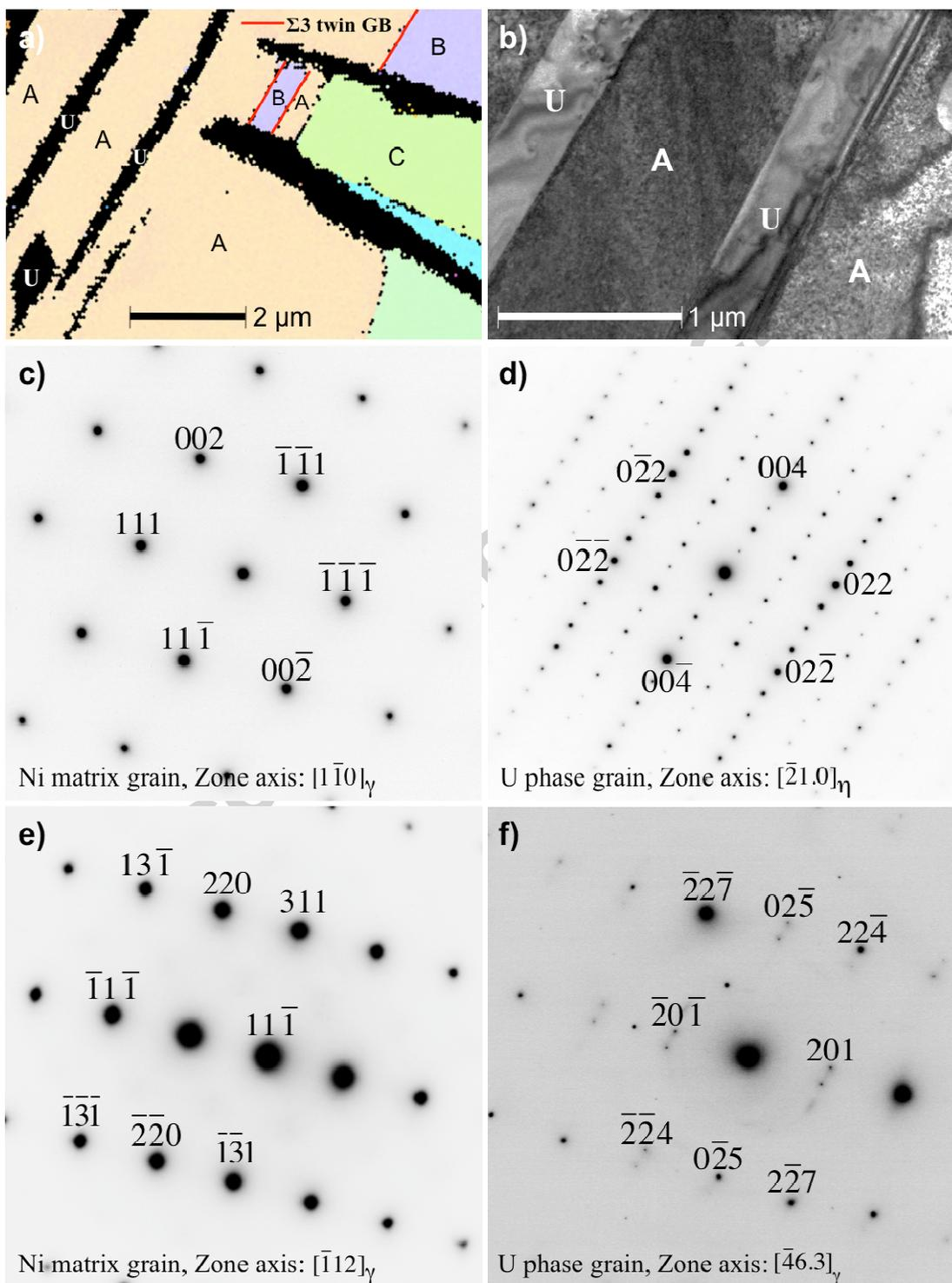
Fig. 3 a) Inverse pole figure (IPF) orientation map of the electron transparent foil; b) the bright field micrograph; c) The  $[1\bar{1}0]_{\gamma}$  zone axis diffraction (ZAD) pattern taken from grain A; d) The  $[\bar{2}1.0]_{\eta}$  pattern of the U phase grain at the same specimen tilts as c); e) The  $[\bar{1}12]_{\gamma}$  diffraction pattern taken from grain A; d)  $[\bar{4}6.3]_{\eta}$  ZAD pattern of the U phase grain at the same specimen tilts as e);
