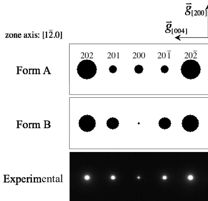
Fig. 12 Comparison of the relative intensities of the simulated and experimental reflections of the row  $[20n]^*$  in the  $[\bar{1}2.0]$  ZAD patterns.
