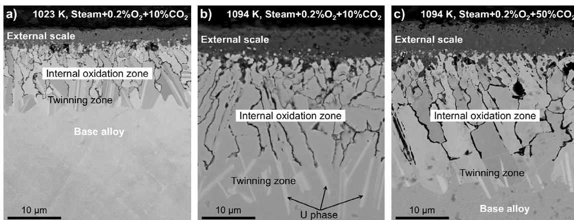
Fig. 1 Backscattered electron (BSE) image of cross-sections of Inconel 939 alloys after 1000 hours of isothermal oxidation at a) 1023 K, b) 1094 K and c) 1094 K in a higher CO<sub>2</sub> percentage atmosphere.
