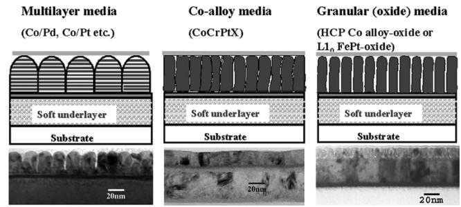
Fig. 1. Schematic structures and cross section microstructures of three types of perpendicular media.
