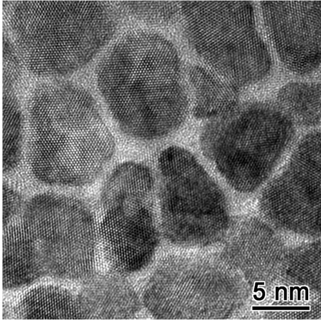
Fig. 4. HRTEM of a Co based granular media with grain size of about 5 nm. This media displays high coercivity and has good grain to grain magnetic isolation due to the continuous film of oxide at the Co boundaries.
