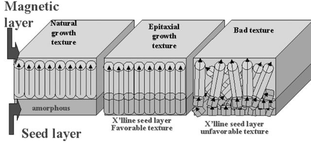
Fig. 2. Schematic representations of the growth of Co grains on different intermediate layer structures.
