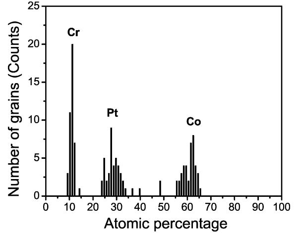
Fig. 6. Composition variation of grains in a nominal Co-11Cr-28Pt thin film. Note that the Cr composition has a narrower distribution than the Pt distribution.
