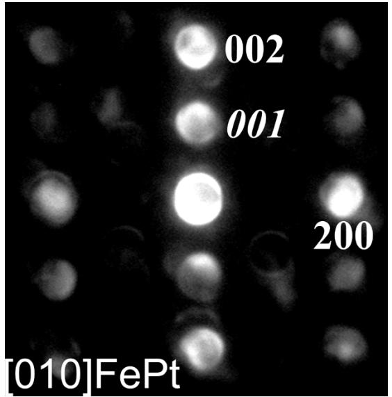
Fig. 7. A nano beam electron diffraction pattern of  $L1_0$  FePt thin film taken in cross section. The film has perpendicular texture.
