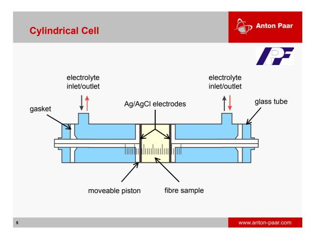
The measuring cell consists of a glass cylinder with inlet and outlet tubes for the electrolyte solution. The fibre sample is mounted between a pair of perforated Ag/AgCl disc electrodes. The electrodes are mounted onto moveable pistons which allow a variation of the distance between these electrodes and therefore an adjustment of the packing density of the fibre sample.
