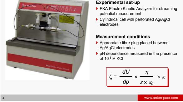
The streaming potential experiments were carried out with the Electro Kinetic Analyzer using the Cylindrical Cell, which was developed for the measurement of fibrous samples, but also for the measurement of granular and powder samples. For each measurement, an appropriate fibre plug was placed between the Ag/AgCl disc electrodes of the Cylindrical Cell. The pH dependence of the zeta potential was investigated with the background electrolyte of 1 mM KCl solution.
