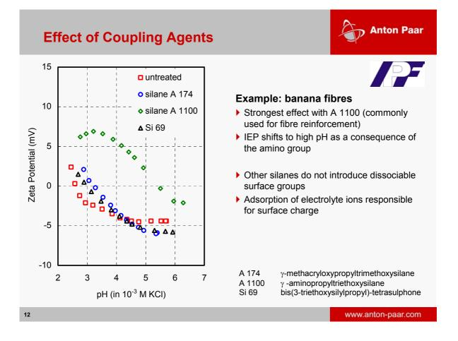
The pH dependence of the zeta potential of banana fibres treated with different silane coupling agents is shown in this graph.
