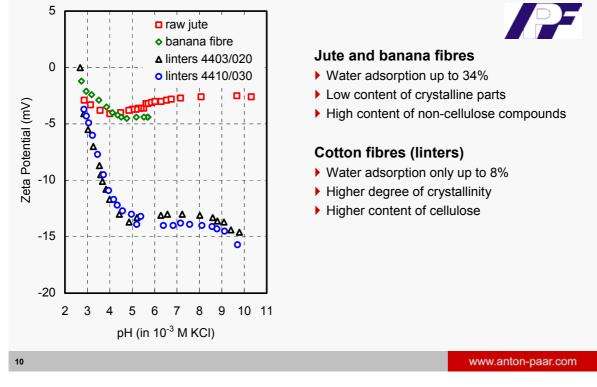
The pH dependence of zeta potential for various natural cellulose-based fibres is shown in this graph.
