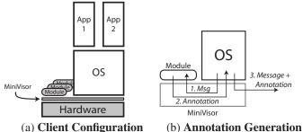
Figure 2: Client Operations. (a) The client attests to a protective layer (MiniVisor) that isolates modules from untrusted code (and vice versa) and from each other. (b) Untrusted code submits messages (e.g., email or packets) to the modules to obtain authenticated annotations.
