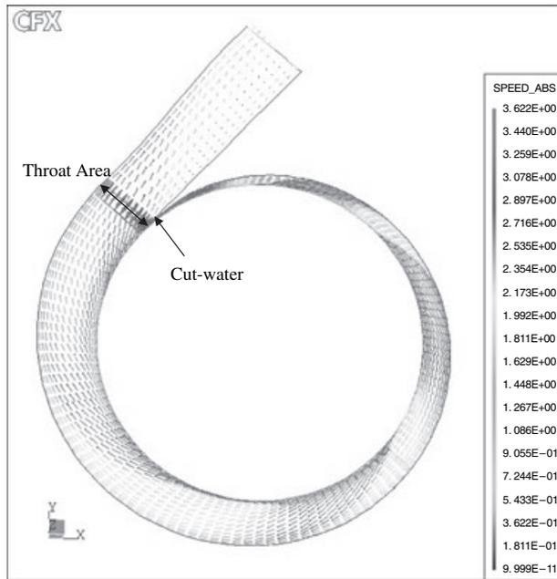
FIG. 5. Velocity profile in the exit volute.
