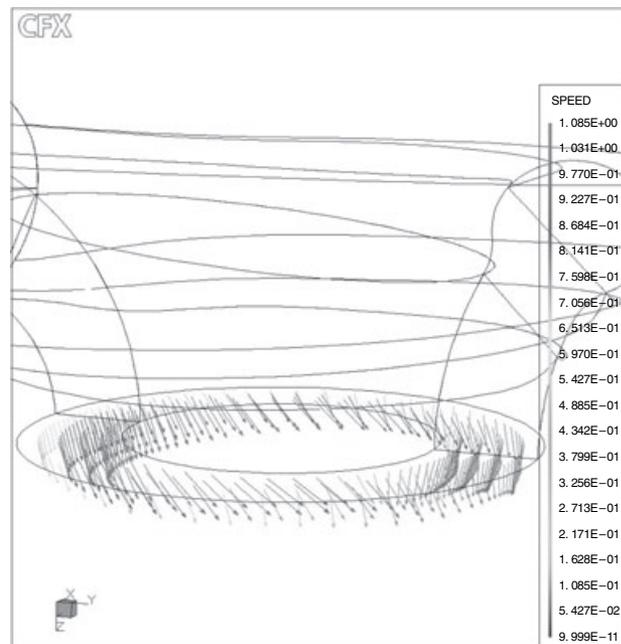
FIG. 4. The velocity profile at the outlet of the flat inlet elbow.
