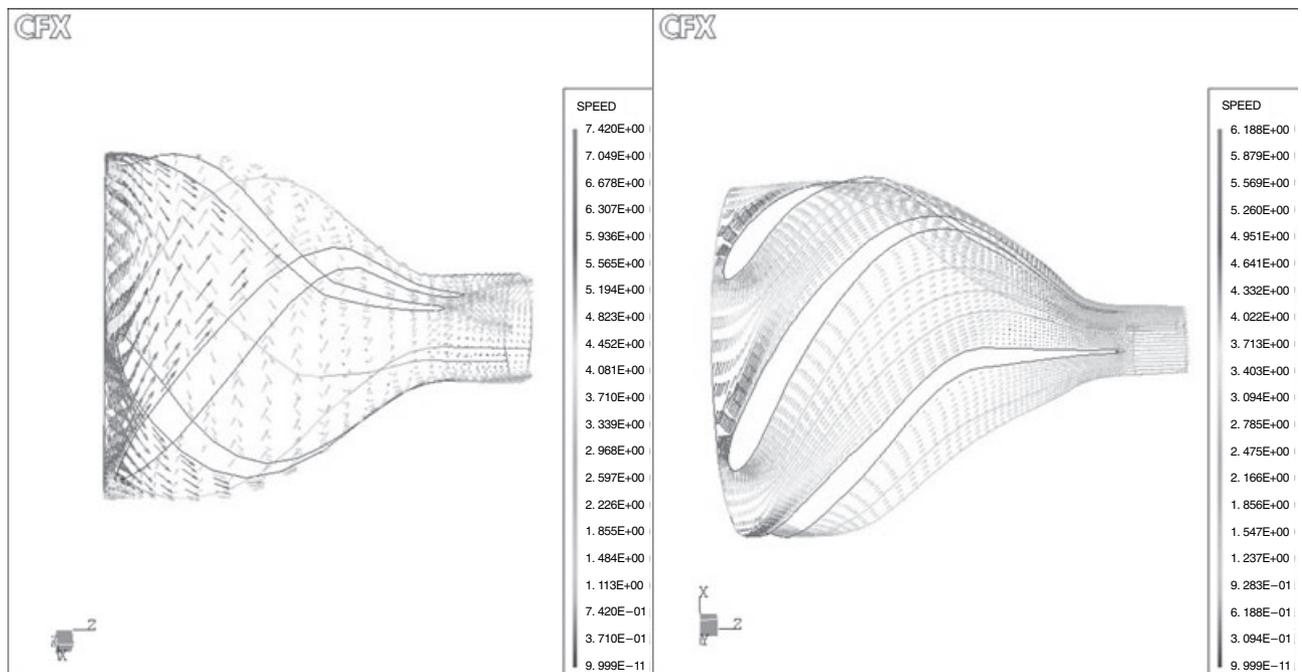
FIG. 6. The comparison of velocity profile in diffusers with different blade numbers.
