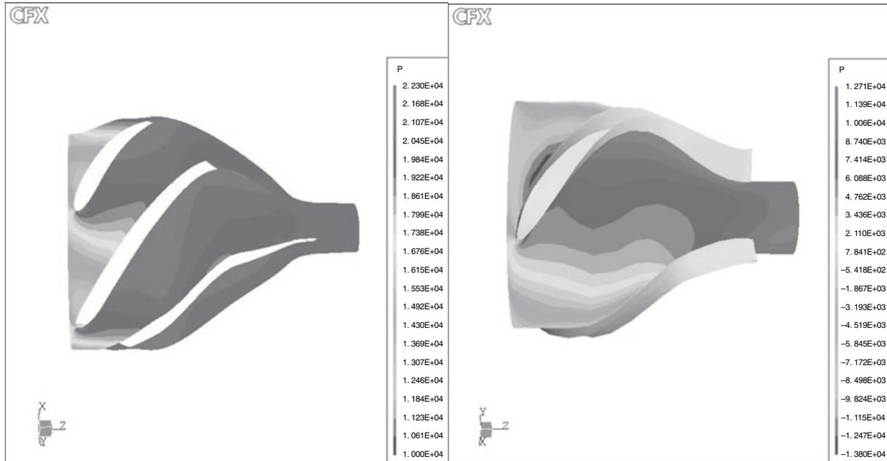
FIG. 7. The comparison of pressure distribution in diffusers with different blade numbers.
