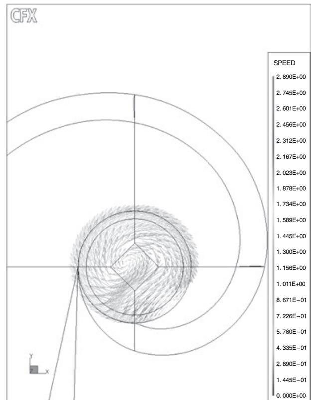
**FIG. 2.** The velocity profile at the outlet of the inlet volute.
