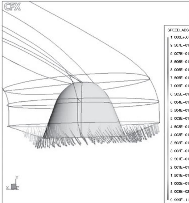
FIG. 3. The velocity profile at the outlet of the inlet elbow.
