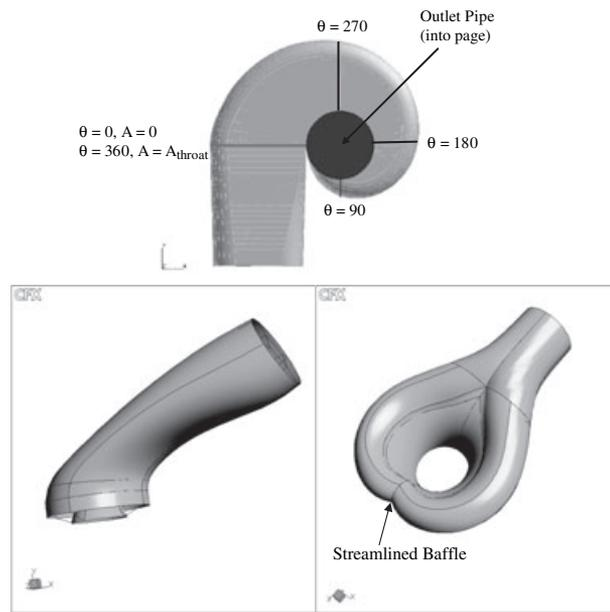
**FIG. 1.** The geometries of different inlet devices for centrifugal blood pumps.
