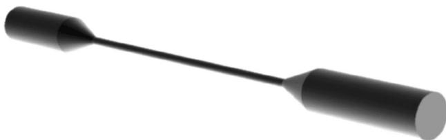
**Figure 2.** Solid model of capillary tube for CFD analysis. The test segment is 1 mm diameter and 70 mm length and is fitted at each end with conically shaped connectors 8 mm length.
