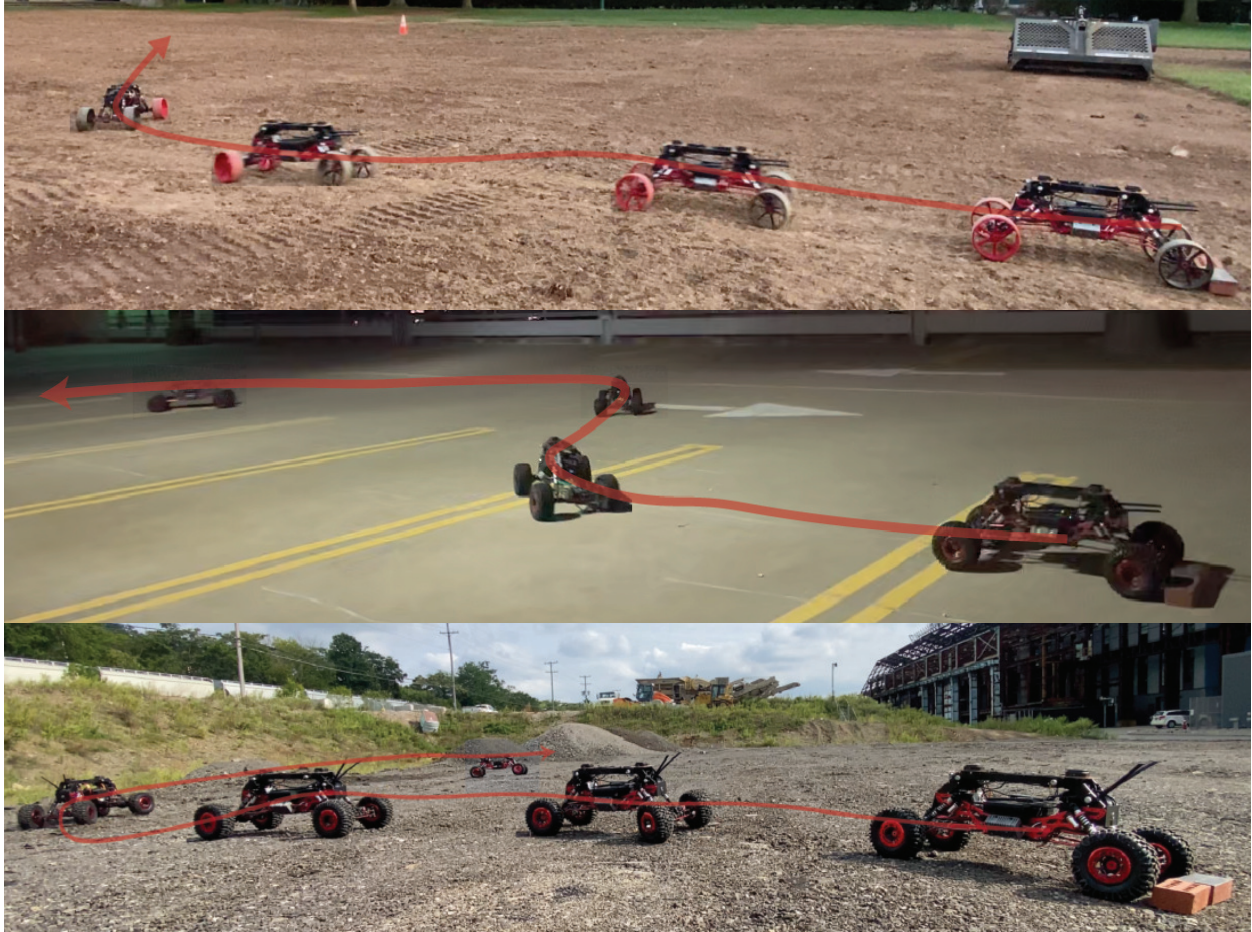
Figure 4.4: Sim2real Experiments. From top to bottom, the wheeled robot driving on dirt, concrete, and gravel. The red line indicates the predefined track for each trial. The tires were changed from compliant rubber tires to hard plastic tires in the dirt experiment shown.
