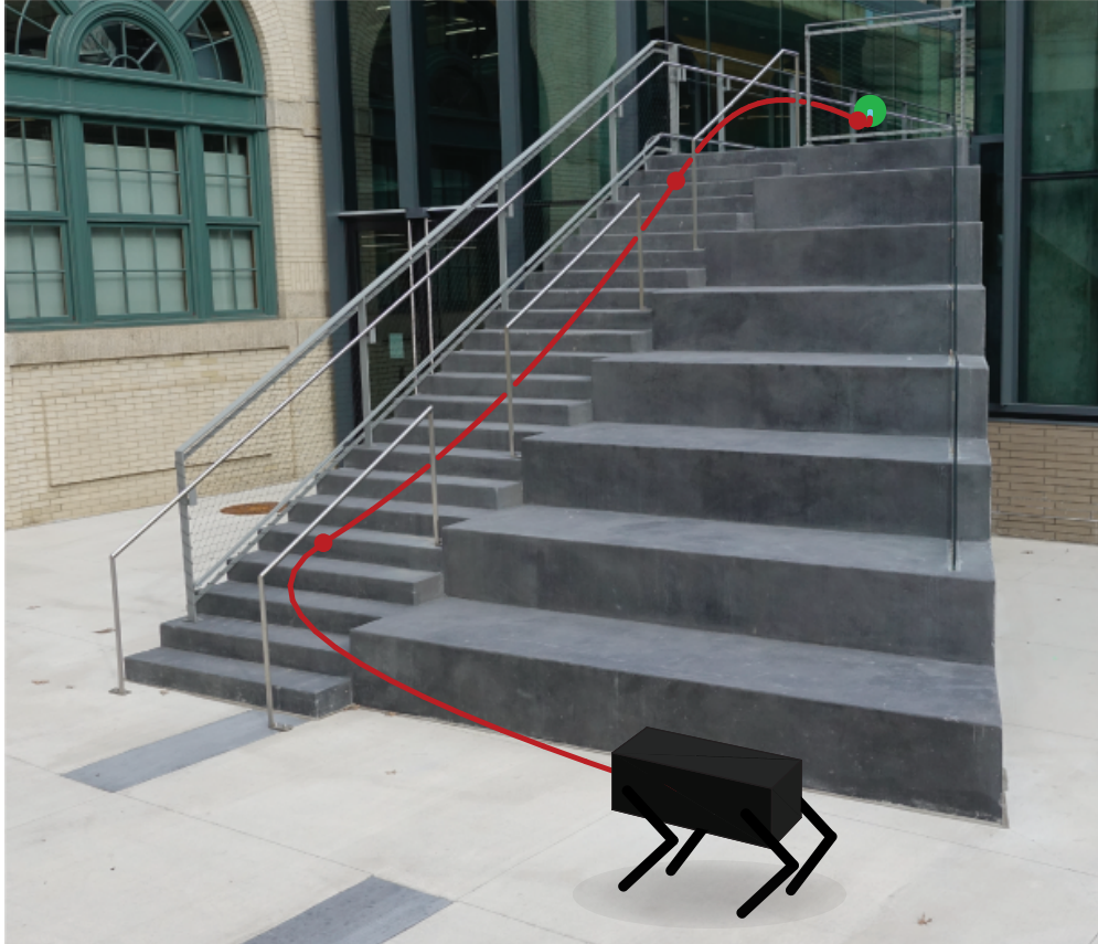
Figure 4: Demonstration of the proposed algorithm generating a long dynamical plan over terrain challenging for a legged robot in under three seconds. The trajectory from the start pose to the goal (green circle) is overlaid on an image of the environment used to generate the plan.
