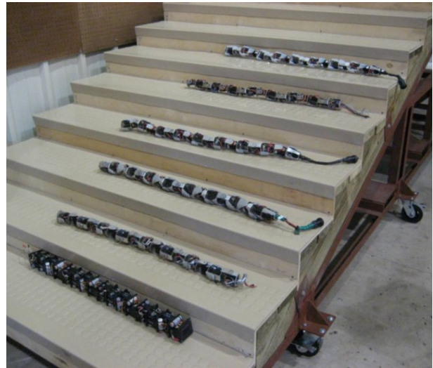
Fig. 2. Progression of modular snake robot development - older robots are at the bottom of the image.
