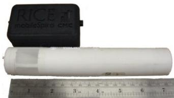
**Figure 1** - mobileSpiro sensor and laminar flow tube
