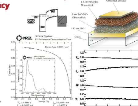
The device polarity can also be switched (where holes now get collected at the back electrode). This removes the 'dead' region. Using small PbS (1.3 eV) a device with 2.94% NREL certified efficiency was obtained. The device is also relatively stable in air. We show a plot of the PV parameters with 1000 hr degradation study in air. The efficiency retains 85% of the starting value.
