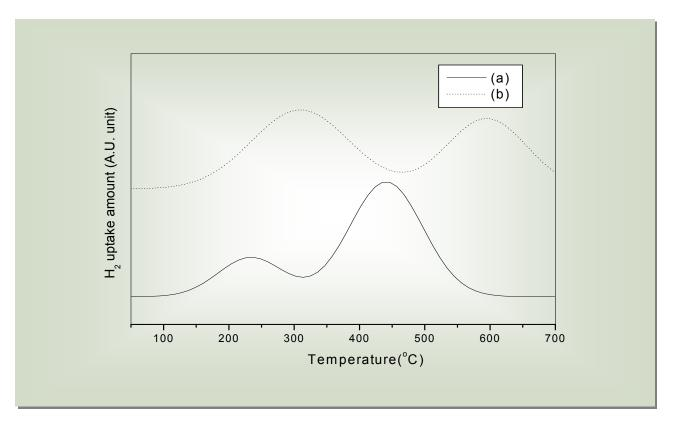
Temperature programmed reduction of  $La_{0.8}Sr_{0.2}Mn_{1-x}O_3$  powder after calcination 1000 °C for 4hrs with different starting Materials. (a) nitrate and (b) Oxide
