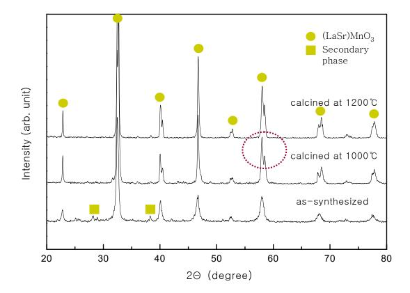
It has single phase after calcination at 1200 °C for 4hrs.
