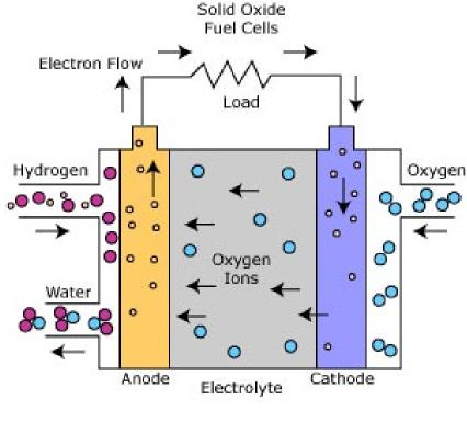
Anode :  $H_2+O^{-2} = H_2O + 2e^{-2}$ Cathode :  $1/2O_2 + 2e^{-2} = O^{-2}$ Total :  $H_2 + 1/2O_2 = H_2O$  Solid oxide fuel cell is energy conversion device that produces electricity by electrochemical. It operate at high temperature over 600 °C with pollution-free technology.
