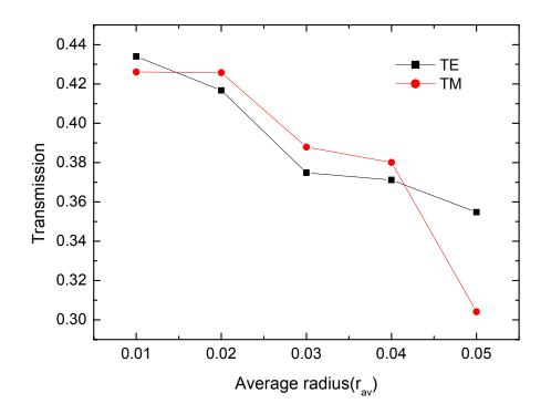
Transmission efficiency as a function of the average radius of nano-particles( $r_{av}$ ).  $a_{av}$  is adjusted at every point so that the simple average index is 2.0.
