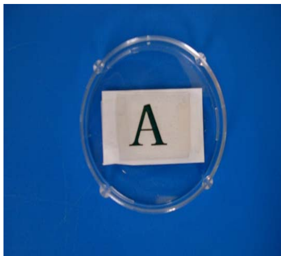
Neat UV-cured PU film
