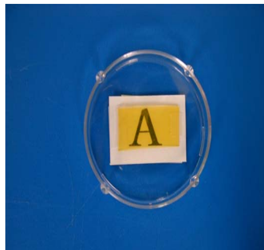
PU film containing CdS nanoparticles
