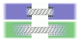
Optimizing the contact between a nanotube and a metal lead
