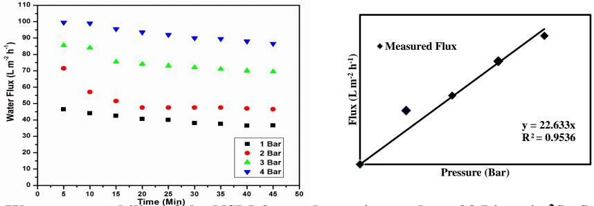
Water permeability of the NSM-2 membrane is equal to ~23 Liters/m<sup>2</sup>/hr/bar.
