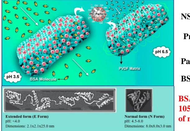
NSM-2 UF Membrane Pressure = 1 bar Particle loading: 38 wt% BSA rejection: 90% BSA binding capacity;
