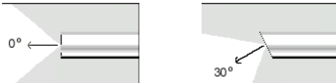
picture 08: Laparoscope Ø 10 mm, 30°, l=310 mm
