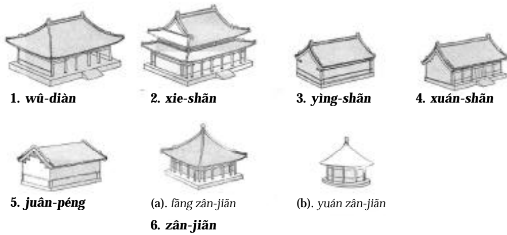
Figure 19. Various types of roofs. (After Lin, 1990: 88)
