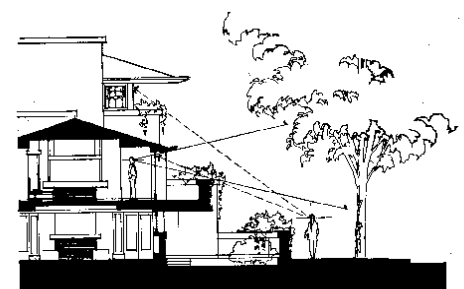
FIGURE 93. Robie House. Living area, showing the dining area beyond. Stairs to the left rear lead to the bedrooms above on the third floor. Cross section and plan indicate the elaborate devices for environmental control that Wright built into the Robie House. Roof overhangs give sun control (1). Ventilation comes from open windows (2) and from glazed doors (3), while the parasol effect of the roof overhangs permits ventilation even during rain storms. Hot air is also extracted from the interior by rising through the lighting grilles into the open space under the roof (4), there to be exhausted through a duct at the side of the main chimney. Concealed heating originates in radiators built into walls under windows (5), or sunk beneath brass floor grilles inside the glazed doors (5). Lighting, too, is integral with the architecture: from exposed spherical globes (7) projecting into the room from the lower edge of the dropped ceiling enclosure for the steel I-beams (8) that support the extensive span and cantilever of the principal roof, as well as from dimmer-controlled lights (9) recessed behind ceiling grilles (10). All opening doors and windows are fitted with screens behind the windows as insect barriers (11).
