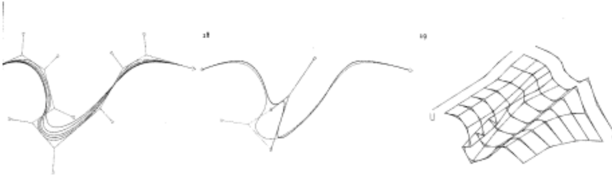
Figure 17: A superimposed series of splines sharing the same control vertices with different degrees of influence; a two-, three-, four-, five-, six-, and seven-degree spline curve.
