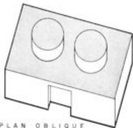
OBLIQUE DRAWING TRUE SHAPE AREAS EMPHASISED AND SHADED
