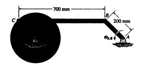
Equation of Motion: Rod BC will always remain in the horizontal and move along a curvilinear path. The acceleration of its mass center G is the same of that for point B and C, i.e.  $a_C = a_C = a_B = \omega_{AB}^2 r_{AB} = 5^2 (0.2) = 5.00 \text{m/s}^2$ . When  $\theta = 0^\circ$ , the acceleration is directed vertically downward. From FBD(a), we have
