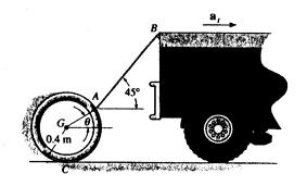
17-51. The uniform connecting rod BC has a mass of 3 kg and is pin-connected at its end points. Determine the vertical forces that the pins exert on the ends B and C of the rod at the instant (a)  $\theta = 0^{\circ}$ , and (b)  $\theta = 90^{\circ}$ . The crank AB is turning with a constant angular velocity  $\omega_{AB} = 5$  rads/s.
