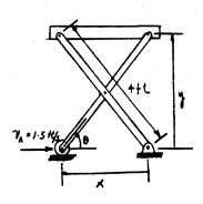
16-43. The end A of the bar is moving to the left with a constant velocity  $\mathbf{v}_A$ . Determine the angular velocity  $\boldsymbol{\omega}$  and angular acceleration  $\boldsymbol{\alpha}$  of the bar as a function of its position x.
