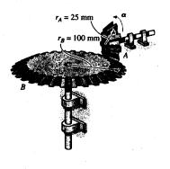
**16-25.** The disk starts from rest and is given an angular acceleration  $\alpha = (10\theta^{1/3})$  rad/s², where  $\theta$  is in radians. Determine the magnitudes of the normal and tangential components of acceleration of a point P on the rim of the disk when t = 4 s.
