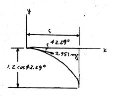
14-95. A 2-lb block rests on the smooth cylindrical surface at A. An elastic cord having a stiffness of k = 2 lb/ft is attached to the block at B and to the base of the cylinder at C. If the block is released from rest at A, determine the longest unstretched length of the cord so the block begins to leave the cylinder at the instant  $\theta = 45^{\circ}$ . Neglect the size of the block.
