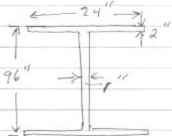
By symmetry (top and bottom), can see that the centroid is in the center.
