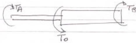
$$\sum M_x = T_0 - T_A - T_B = 0 \Rightarrow T_A + T_B = T_0 \quad \text{static.}$$
