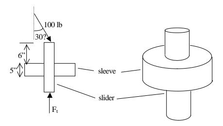
Take the fit between the slider and the sleeve to be such that there is contact at only two points. The slider is moving steadily (no acceleration) and kinetic friction prevails.
