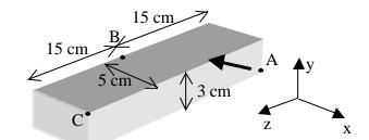
**2.** (**20 points**) The body shown is subjected to two forces and it is maintained in the position shown by a hand which firmly grips the handle at A. The 25 lb force accounts for the weight. The 10 lb force is applied in the middle of its face. The handle comes out from the middle of its face.
