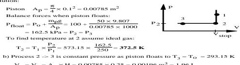
$V_2 = V_1 = A_p \times H = 0.00785 \times 0.25 = 0.00196 \text{ m}^3 = 1.96 \text{ L}$
