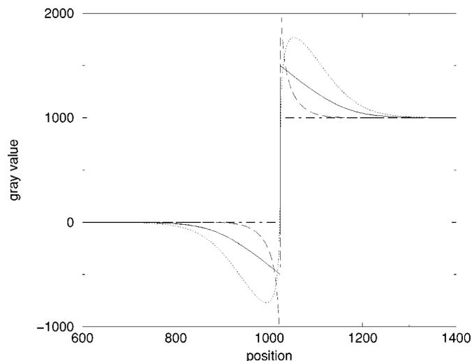
Fig. 17. Response of Laplacian Pyramid-based enhancement with varying gain to a step edge. The remapping function was linear. Dotted-dashed line: original edge; full line:  $g_0 = \dots = g_6 = 2.0$ ; long-dashed line:  $g_0 = 4.0, g_1 = 3.5, g_2 = 3.0, g_3 = 2.5, g_4 = 2.0, g_5 = 1.5, g_6 = 1.0$ ; dotted line:  $g_0 = 1.0, g_1 = 1.5, g_2 = 2.0, g_3 = 2.5, g_4 = 3.0, g_5 = 3.5, g_6 = 4.0$ .
