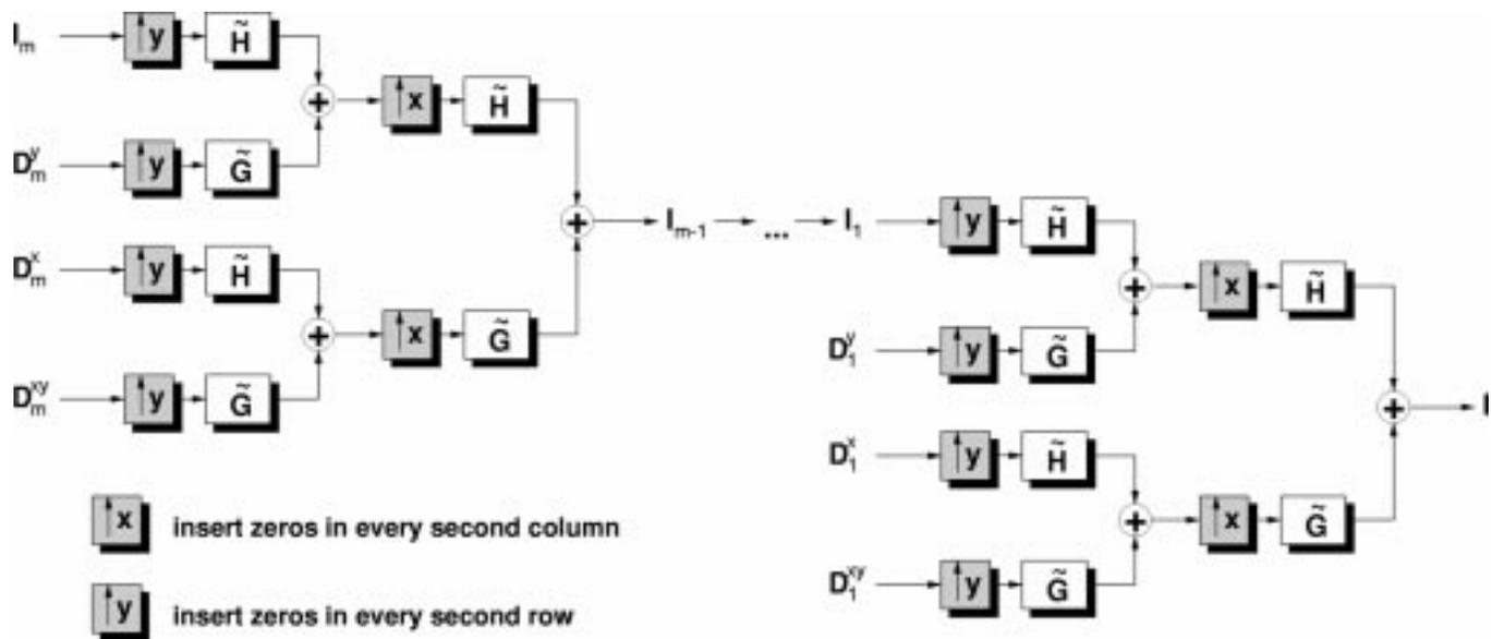
Fig. 3. Filter bank representation of the back transformation corresponding to the decomposition shown in Fig. 2.  $\tilde{H}$  and  $\tilde{G}$  denote the inverse filters of  $H$  and  $G$ . Though in the orthonormal case,  $\tilde{H} = H$  and  $\tilde{G} = G$ , in more general cases, e.g., for biorthogonal wavelets as discussed below, they may differ.
