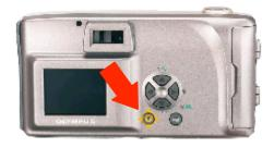
2. To make a preview appear in the screen on the back, press the bottom-left button on the back.
