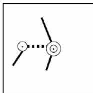
Fixed (the dashed line is constrained to be horizontal)
