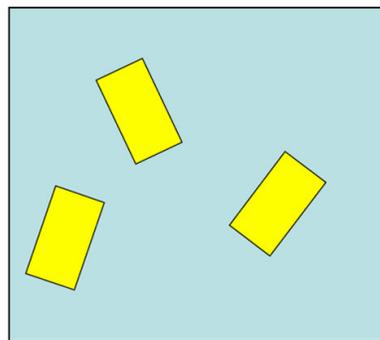
Allowed to move in  $x$  and  $y$  and to rotate: 3DOF ( $x, y, \theta$ )
