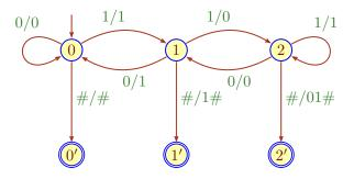
Lastly, a machine that assumes that every track has a special endmarker #. Note that this machine is clearly deterministic, the endmarkers tell us when the end of the input has been reached.
