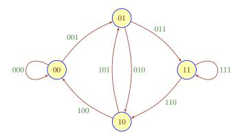
Each configuration in  $2^{\mathbb{Z}}$  corresponds to exactly one biinfinite path in this automaton. And every biinfinite path corresponds to a configuration (at least if we are a bit relaxed about where the origin is).
