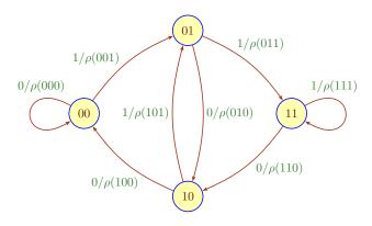
If we replace the edge labels xyz by  $xyz/\rho(xyz)$ , where  $\rho$  is the local rule, we get a transducer that corresponds to the global map. All states are initial and final, we are interested in biinfinite runs.
