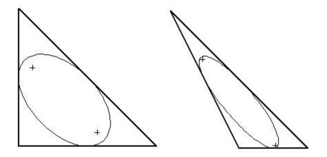
Joe knows how to draw an ellipse by putting two stakes in the ground (at the foci of the ellipse), tying a rope between them and dragging a marker stick inside the rope. What Joe would like is for the customer to determine where the corners of the triangle will be and then measure the location of the triangle vertices and compute where to put the stakes and how long to make the rope.
