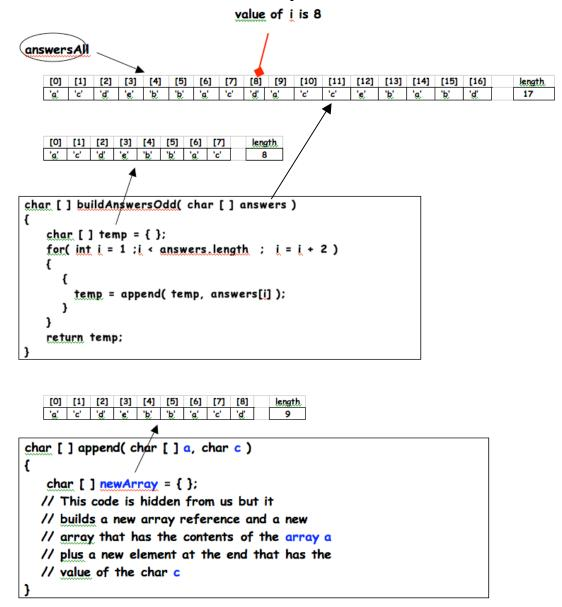
The next page shows the structure of the arrays after the **append()** function has returned the reference to the new array:
