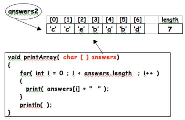
For the second call where the argument is answers2, Processing assigns the argument, answers in the definition to reference the same array as answers2. When it needs to know the length of the array, it follows the arrow to the array and finds the length of this array to be 7.
