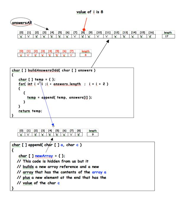
The array reference temp is no longer pointing to the 8 element array now shown in red. It is pointing to the new array that contains all of the elements in the old array plus one more - the value of element [8] in the array referenced by answers. The old array now shown in red that temp used to reference now has no references. We can no longer access any of the values stored in it. It is lost to us forever.<sup>1</sup>
