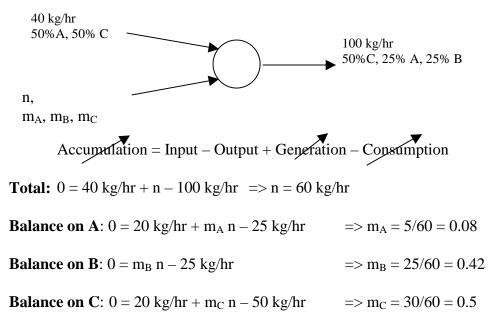
So, the unknown stream flows at 60 kg/hr and is 8%A, 42% B and 50% C
