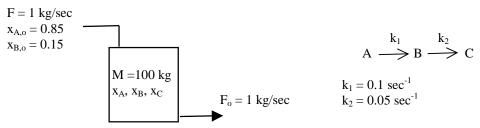
The total mass of material in the reactor is constant at M = 100 kg and the concentrations are in terms of mass fractions (i.e.,  $x_A$  [=] gm A/gm total). The reactions are first order such that mass consumed = k  $x_{reactant}$ .
